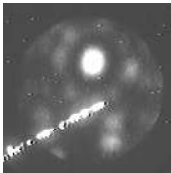
Figure 4.18: FIM picture of a polycrystalline tungsten tip which is so sharp that only a few atoms are imaged; the ring counting method is thus impossible to apply for this tip apex. This FIM image was acquired at room temperature, at a BIV of 2.4 kV.
